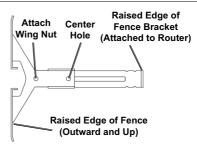
Figure E: Circle Cutting with Fence
