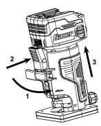
Figure A: Router Bit installation
