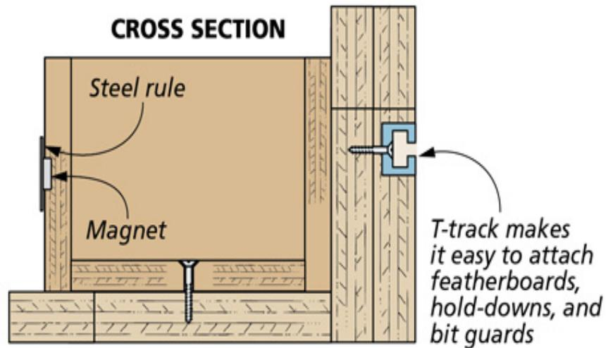
I used screws to fasten the trays to the base. A couple of small rare-earth magnets on the back hold a steel rule I use for setup.
