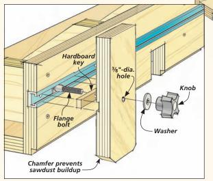
**STOP BLOCK.** A stop block, like the one you see in the drawing at left, is a handy accessory to add to your router table fence. It allows you to make repetitive cuts quickly and accurately.
