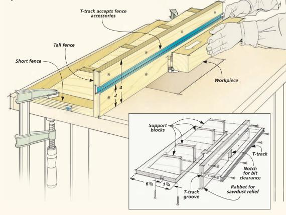
face of each piece and install the T-track in the groove.
