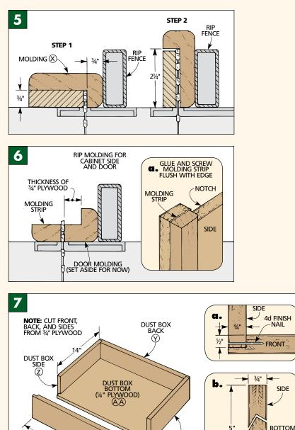
and add  $7/_{16}$ " to each measurement to account for the grooves. Cut the bottom from  $1/_4$ " plywood.
