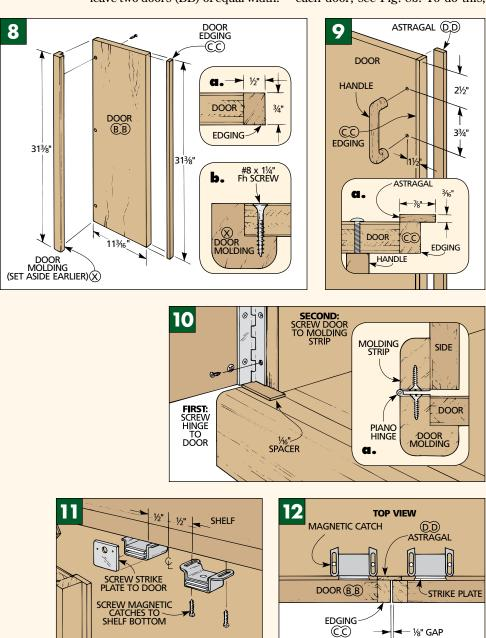
drill countersunk shank holes from the back side of each door centered  $\frac{3}{8}$ " from the outside edge. Clamp the molding in place and drill pilot holes into the molding. Then glue and screw a molding strip to each door using #8 x  $\frac{1}{4}$ " Fh woodscrews.
