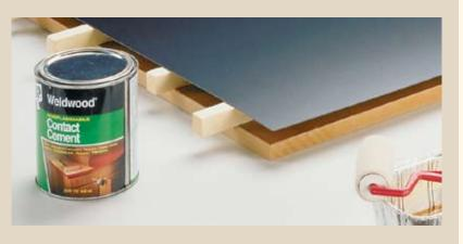
JOINING THE PIECES. The contact cement has to be almost dry before joining the two pieces. You can check it by simply dabbing it with your finger. It should look dull and feel slightly tacky, but shouldn't stick to your finger.
