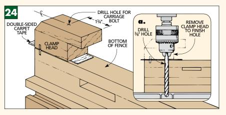
long enough to drill through both pieces at once, drill as deep as you can. Then remove the clamp head and continue on through the fence to finish the hole; see Fig. 24a.
