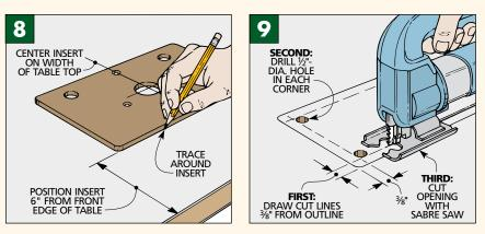
**22** Remove the insert plate, but don't cut the opening yet. First, lay out lines for the recessed lip that will hold the insert plate. To do this, draw lines  $\frac{3}{8}$ " in from the plate outline; see Fig. 9.
