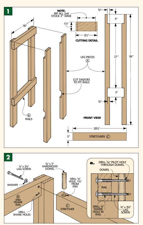
**9** Place a stretcher (C) against a rail. Drill a  ${}^{3}/{}_{16}{}^{"}$ -dia. pilot hole through each shank hole into the stretcher and through the dowel in the stretcher; see Fig. 2. Repeat this process to drill pilot holes into all the stretchers.
