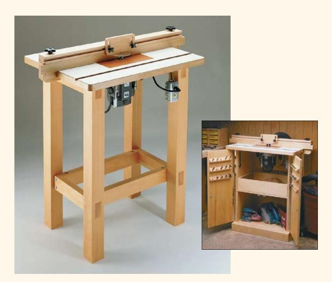
A router is one of the most versatile tools in the shop. Mount it in a router table, and you'll find dozens of new uses for this tool.
