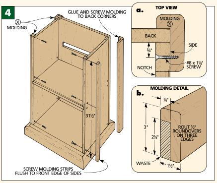
the inside face of the case sides and back; see Fig. 3. Next, drill pilot holes into all four base pieces. Finally, glue and screw the base pieces in place using  $#8 \times 1^{1}/_{4}$ " Fh woodscrews.
