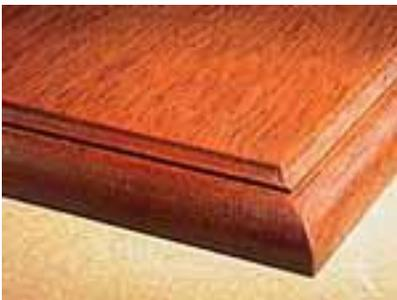
When applying liquid stains, the stain soaks more deeply into the pores of the end grain than the face grain, darkening the ends much more than the faces, see top photo.
