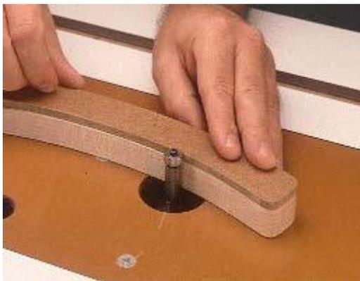
One of the simplest ways to duplicate curved parts is to use a template and a flush trim bit, see photo. It's quicker and more accurate than roughing out the shape on a band saw and sanding up to a layout line — especially when you're making multiples.
