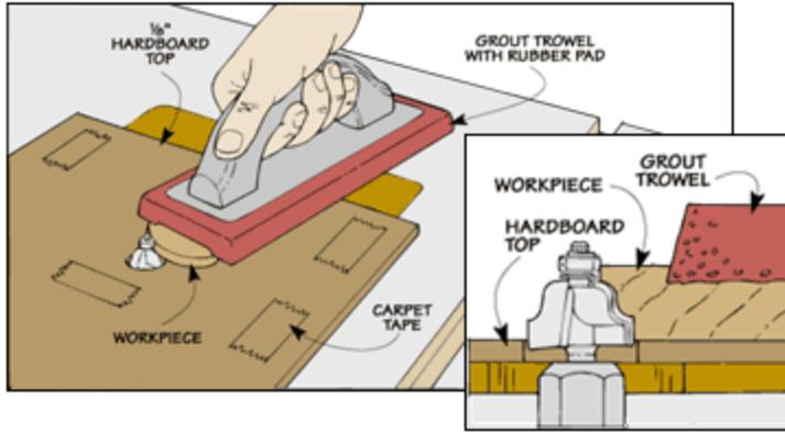
One solution is to add an auxiliary top made of 1/8" hardboard. To provide clearance for the router bit, you'll need to drill a hole in the top. Note: Drill the hole slightly larger than the bit.
