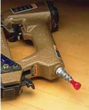
Dust and dirt can cause the seals of air-powered tools to wear out too quickly. To protect my brad and nail guns from sawdust and debris when they're not being used, I simply plug the air inlet holes with golf tees.
