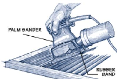
Hold the stick against the pad of your palm sander. Next, place a size 84 rubber band (available at office supply stores) onto the handle indentation of the stick and pull the rubber band up and over the edges of your sander. Hook it onto the other end of the stick. When
