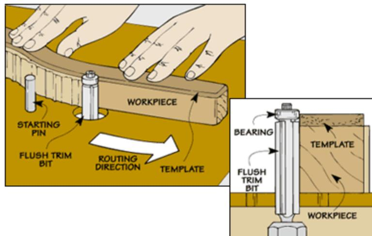
To make a template, start by laying out the shape you want on the hardboard. Or you can cut a full-size pattern out of paper and glue it to the hardboard. Then cut out the shape slightly oversize, and file (or sand) carefully up to the line.
