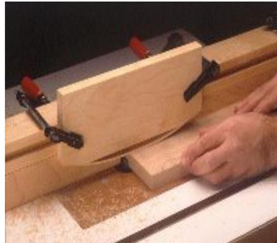
In use, the hold-down is clamped to the fence so enough downward pressure can be applied to the workpiece to keep it flat against the table top — without causing the workpiece to bind.
