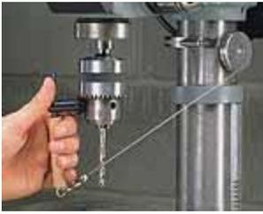
I'm always misplacing the chuck key to my drill press. So I fastened it to a retractable key chain that's attached to the column of the drill press, see photo.
