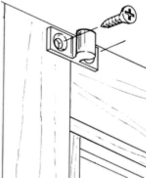
Typically, when installing ball catches, I mount the "strike" part of the catch to the inside of the door first, see Fig. 1. (Make sure the strike is just below the top of the cabinet.)
