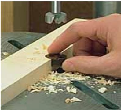
A cam-action knock-down fastener needs to fit tightly in its hole to create a good, tight joint. And the depth of the hole is critical, too. But once the plastic cam is tapped into the hole, it's tough to get it out again to adjust the depth of the hole without damaging the fastener.
