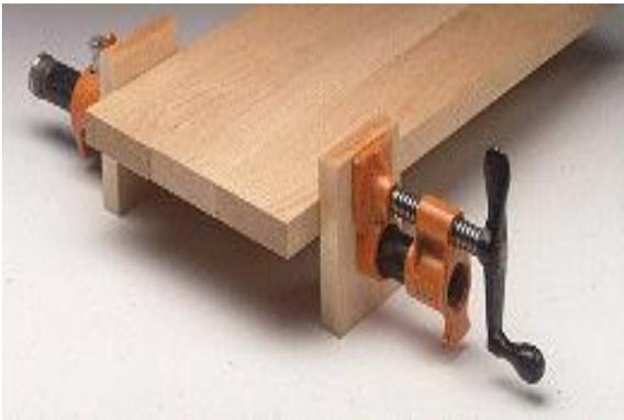
Tightening a pipe clamp can be a real knuckle buster when the pipe clamp sits on the workbench. So I made a couple  $\frac{3}{4}$ "-thick wood spacer blocks to raise the pipe clamps up and make it easy to turn the handle.
