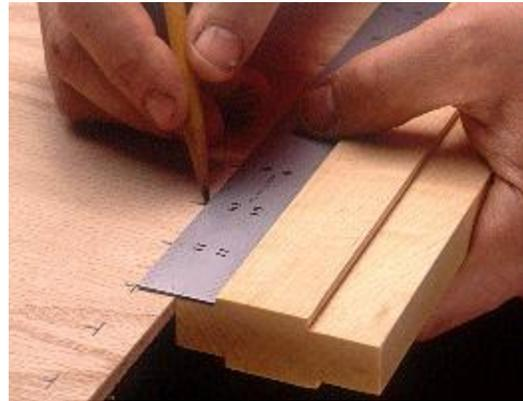
To mark all the screw holes the same distance in from the edge of the plywood back, he mounted a ruler on a piece of scrap wood, see photo. This eliminated the need for a tape measure.
