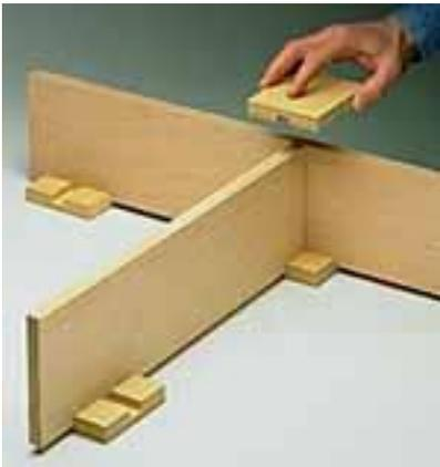
Sometimes you almost need a third hand to assemble a project. Especially working with large pieces of plywood. To help me keep the pieces aligned, I use assembly blocks made from scrap.
