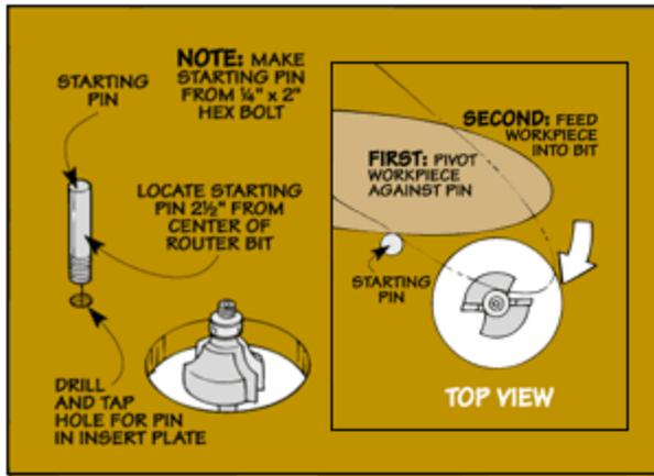
To reduce the chance of that happening, I use a starting pin. This is just a cutoff bolt that threads into a hole in the insert plate.
