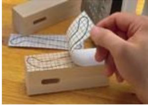
With the photocopy placed face down against the workpiece, slowly move the iron (set on high) back and forth, see top photo.
