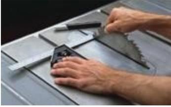
Next, slide the square and rotate the blade backward until the marked tooth aligns with the square. If the square just touches the side of the tooth, the slot and the blade are aligned.
