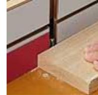
To turn a router table into an edge jointer, simply attach the laminate to the left (outfeed) side of the router fence with carpet tape. The idea is to align one end of the laminate with the opening in the fence, see detail. I also file a bevel on this end to reduce the chance of a workpiece catching on the laminate.
