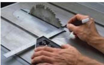
To check that your blade is parallel with the miter gauge slot, first mark a tooth. Then place a square in the slot and adjust it so the end of the square just touches the side of the marked tooth.
