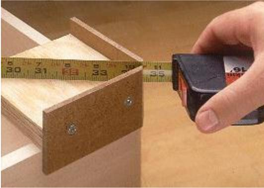
Comparing the diagonals of a cabinet or a box is a great way to check it for square. But when you're working alone in the shop, measuring long diagonals accurately can be difficult. To make this job easier, I made a pair of simple tape holders.
