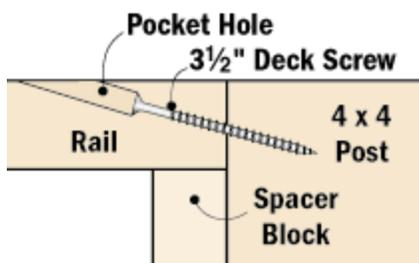
In our *Workbench* [Rustic Retreat Deck](#) project, we needed a quick way to secure  $2 \times 4$  hand rails to the posts. Pocket hole joinery was the perfect solution. We used a pocket hole jig from the [Kreg Tool Company](#) to make sure all the deck screw holes were positioned exactly where we wanted them.
