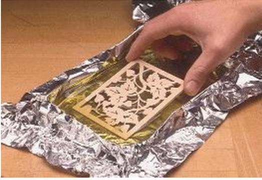
As for applying a finish, we get into the tiny openings by dipping the panel in an oil finish, see photo at right. When dipping a fretwork panel, aluminum foil shaped into a tray acts as a reservoir for the oil finish. To remove the excess finish, you can blot the panel dry with a cloth or blow it out with compressed air.
