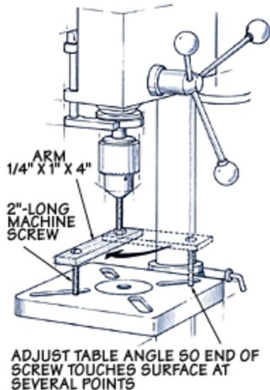
I have a small bench top drill press with a table that tilts to accommodate drilling angled holes, which is very handy. Unfortunately, it doesn't have any stops or markings to let me know when I've got the table set back square to the spindle and bit.
