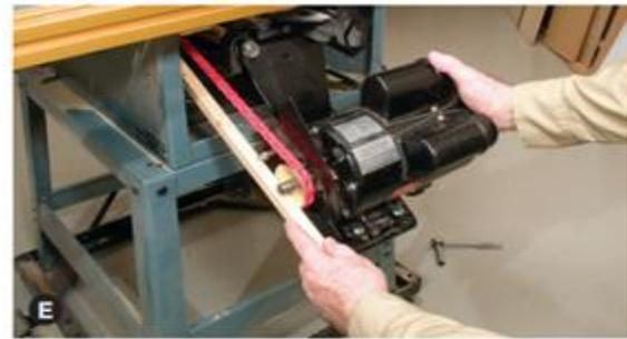
Eliminate vibration and you'll produce improvements at the cutting edge. Align your saw's pulleys and install a Power Twist Link Belt for smooth running.
