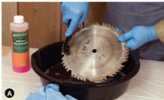
Before you ship the blade off to the sharpening shop, inspect it for a buildup of pitch and resin. You may discover that you have still-sharp teeth hiding under a layer of baked-on residue. Resin Remover, shown in Photo A, is a nontoxic concentrate that you dilute with water and apply by immersing the blade. Save and re-use the cleaning solution until it loses its effectiveness. After you've cleaned, water-rinsed, and air-dried the blade, give it a shot of Dri-Cote
