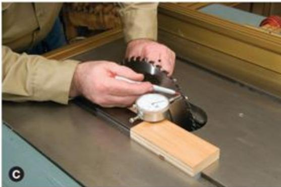
Check the blade's distance from the miter-gauge slot at two positions to make certain that it's parallel.
