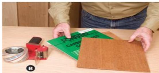
To safely send a blade for sharpening, ship it in its original packaging sandwiched between two pieces of plywood.
