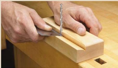
The hardest part of creating a burr on the edge of a scraper is holding the burnisher at a consistent and correct angle. One solution is a simple jig made from a piece of scrap wood and a drill bit, as shown in the photo at left.
