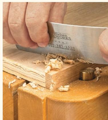
**Plywood Edging.** A scraper excels at leveling edging on plywood without damaging the veneer.
