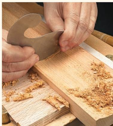
**Saw Marks.** A curved-profile scraper is best to remove saw marks from cove molding made on the table saw.
