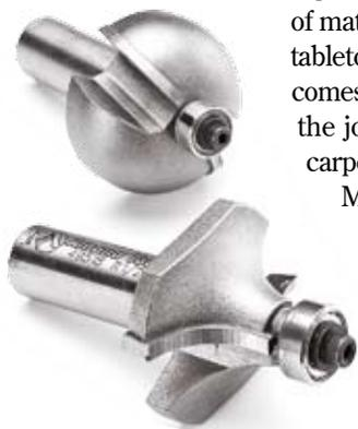
▲ A roundover and a matching cove bit are the start of a rule joint.
