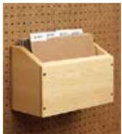
To make it easier to get the sandpaper out of the file, I cut the sides at an angle on the band saw, and then bevel-ripped the top edge of the front on the table saw to match (Figure 20).
