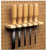
When drilling a hole for a chisel, chamfer the top edge so the ferrule can't slip out (Figures 17 and 17a). When drilling for a screwdriver, counterbore the hole slightly larger than the handle so it sits down into the hole (Figures 18 and 18a).
