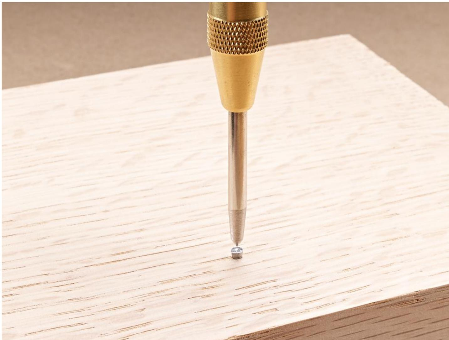
Instead of putting larger holes in trim work using a nail set, *David Fraser* of Modjeska Canyon, California sets the nail heads with an automatic center punch.
