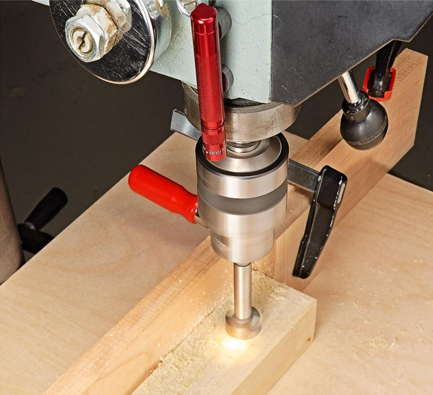
Bill Wells from Olympia, Washington, creates a tiny task light by securing a small metal flashlight to tools with a pair of 1/4"-dia. rare-earth magnets.
