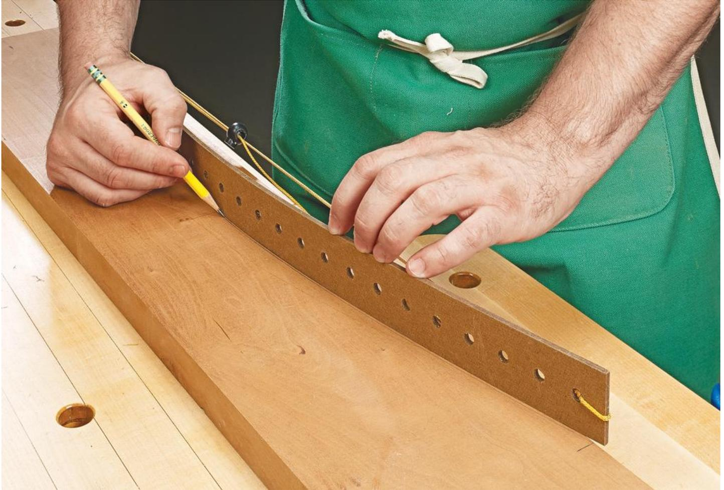
Trying to bend a long, flexible strip and trace an arc at the same time can be tricky. To make it easier, I made an adjustable arc that can be locked into any curved shape I want. The arc is made from a strip of 1/4 pegboard about 24" long, a nylon string and a cord lock that I bought at a fabric store.
