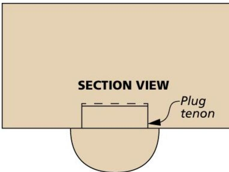
To finish off a small box, sometimes all I need is a simple means to slightly raise the box. I've found that small button plugs work perfect for the job. To install, you only need to drill shallow holes in the bottom of the box for the plugs to slip into. The plugs are then glued in place. And if the box doesn't sit flat, simply run the plugs over a piece of sandpaper on a flat surface to level things out.
