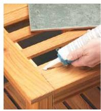
To secure the ceramic tile, put a dot of silicone adhesive toward each end of each spacer, then press the tile firmly into place.
