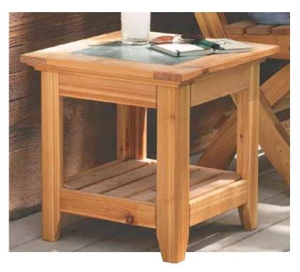
After cutting the stiles to size, you can cut the taper at the bottom of each one, as shown in Figure 1b. Then rout chamfers on the edges with the tapers and also along the bottom edges (Figure 1b).
