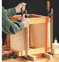
A couple of squaring forms cut from scrap plywood help keep the base square while the band clamps are tightened. Use an exterior-grade glue when assembling
